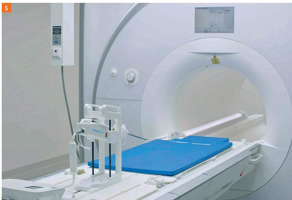
**Figure 5:** TULSA-PRO® system: The ultrasound applicator and robotic positioning system are inside the scanning room on the MRI bed.
