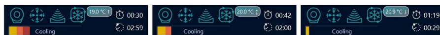
Fig. 20: Three examples of cooling time in the System Status Display. Left: Almost one third of the remaining system-recommended cooling time is mandatory and cannot be overridden. Middle: The cooling period can be overridden because there is no mandatory cooling time, but the system indicates a high risk of internal burn. Right: Recommended cooling time still remaining, but it is possible to use the override and start sonication.
