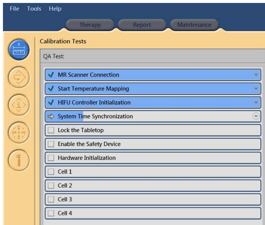
Fig. 109: Automatic QA Test has successfully passed the first three phases and is now performing System Time Synchronization.
