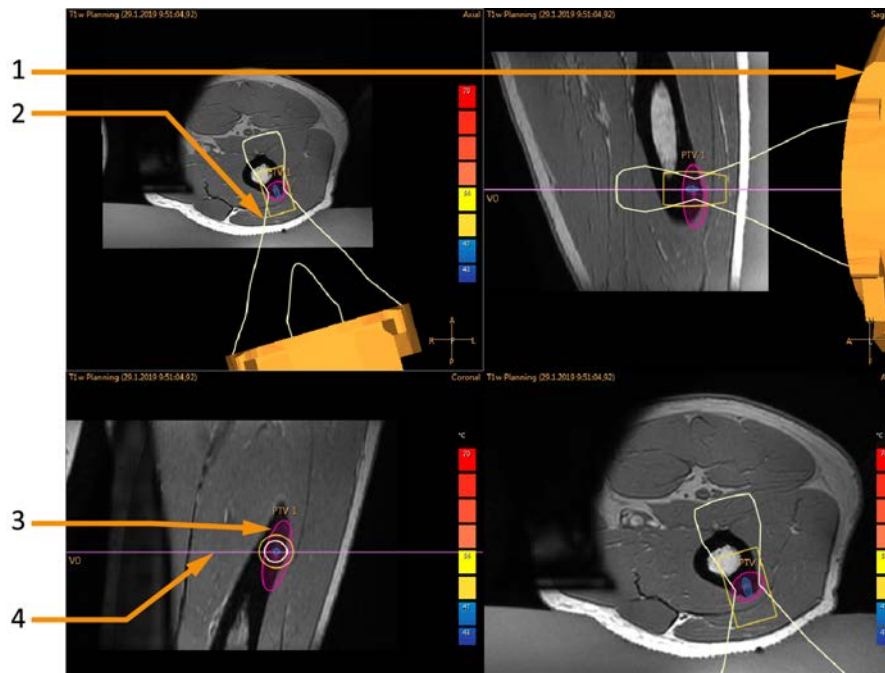
Fig. 34: A number of overlays on top of the transducer view: Transducer overlay (1), Transducer beam overlay (2), PTV overlay (3), View slice overlay (4)
