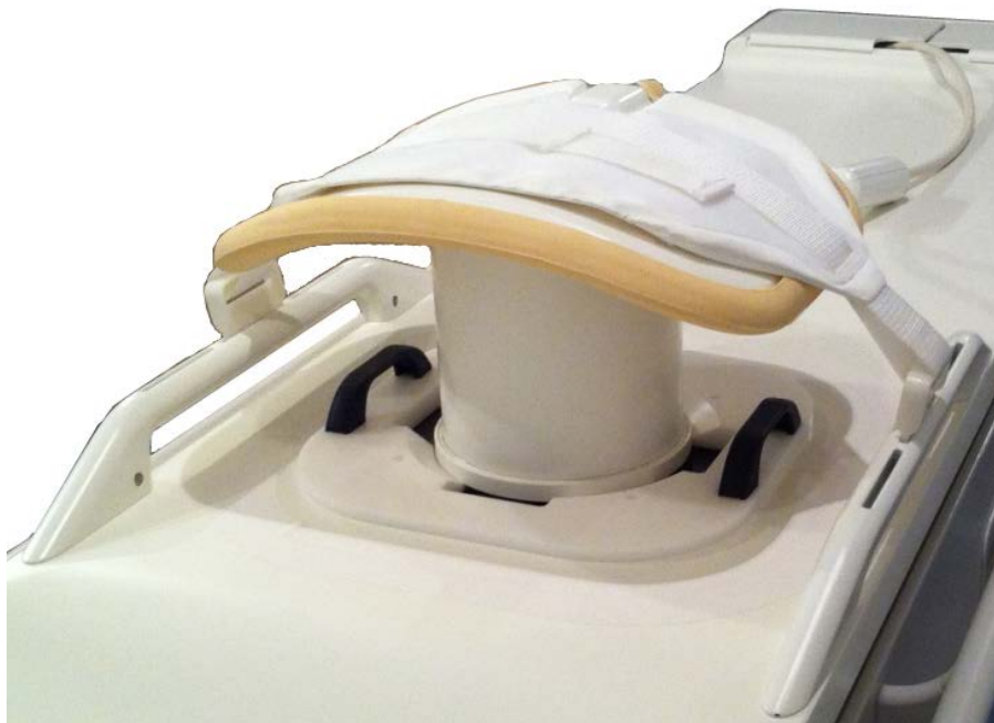
Fig. 109: QA phantom ready for sonication.
