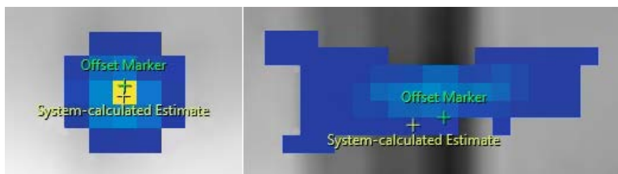
Fig. 89: When you move the offset marker, another marker appears at where the system-calculated estimate was.
