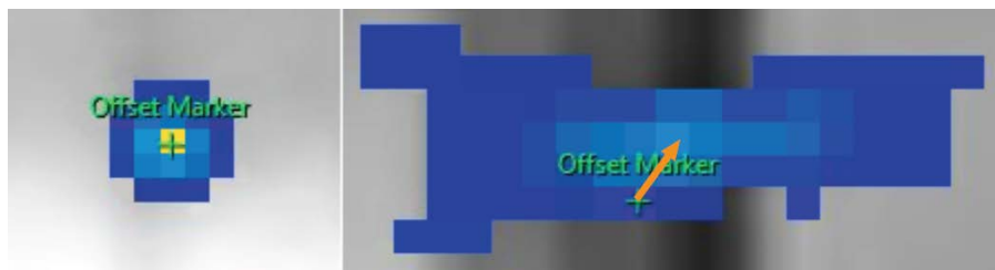
Fig. 88: If the offset marker does not appear at the center of the heating, drag the offset marker to the center of the heating manually.
