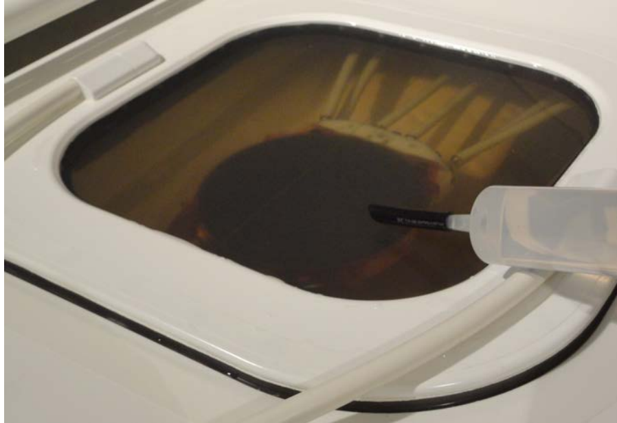
Fig. 110: Preparing the Sonalleve Table Top with degassed water for phantom.
