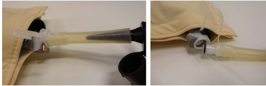
Fig. 118: Releasing the tube from the valve.
