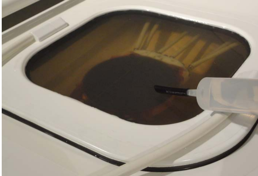
Fig. 101: Preparing the Sonalleve Table Top with degassed water for phantom.
