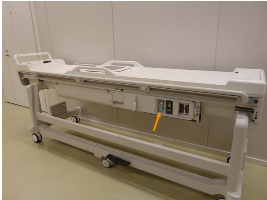
Fig. 5: When DISC is pre-installed at the factory, the hose connectors are located in the Table Top connector panel.
