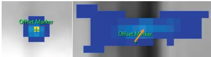
Fig. 87: If the offset marker does not appear at the center of the heating, drag the offset marker to the center of the heating manually.
