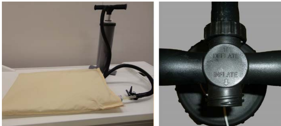
Fig. 116: Air pump. Right: Air hose connected to the Deflate side of the handle.
