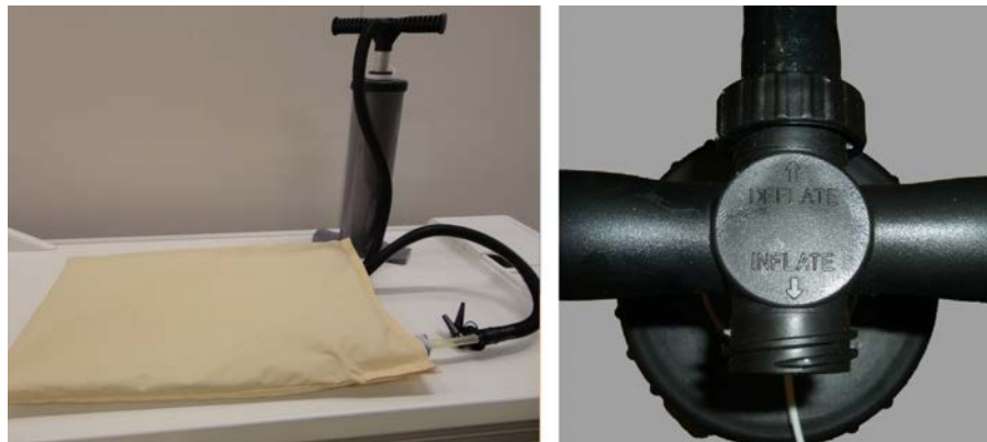
Fig. 119: Air pump. Right: Air hose connected to the Deflate side of the handle.
