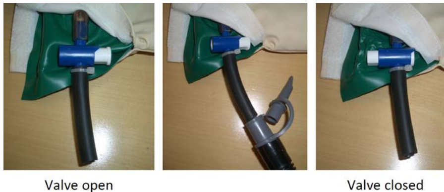
Fig. 122: Another type of valve. Left: the valve is open; middle: the air hose is connected; right: the valve is closed and the air hose has been detached.
