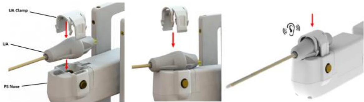
Figure 23: UA attachment to Positioning System
