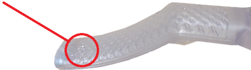
Figure 13: Lubricant emerging from ECD pores
