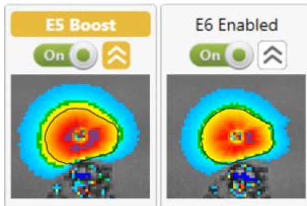
Figure 55: Max temperature maps of the same target boundary treated with boost (left) and without (right).
