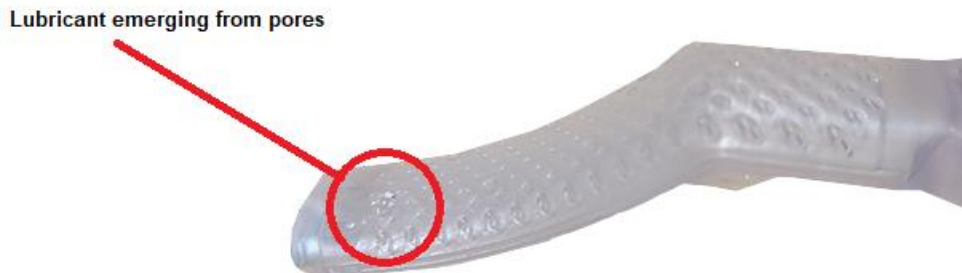
Figure 13: Lubricant emerging from ECD pores
