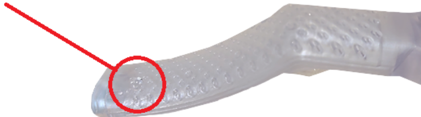
Lubricant emerging from pores
