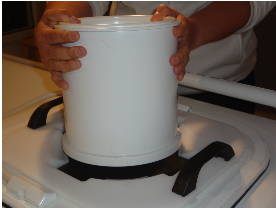
Fig. 109: Place one edge of the QA phantom on the phantom plate. Gently lower the QA phantom onto the phantom plate.
