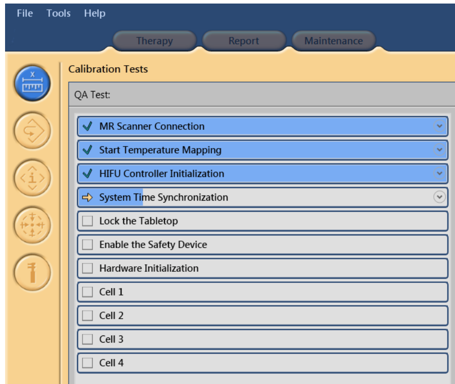
Fig. 114: Automatic QA Test has successfully passed the first three phases and is now performing System Time Synchronization.
