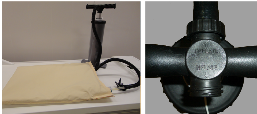
Fig. 121: Air pump. Right: Air hose connected to the Deflate side of the handle.
