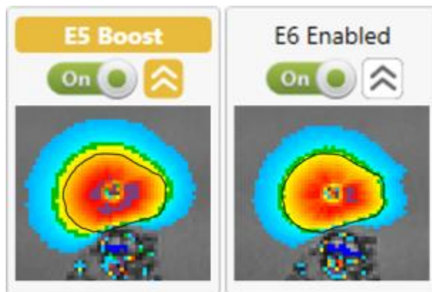
Figure 54: Max temperature maps of the same target boundary treated with boost (left) and without (right).
