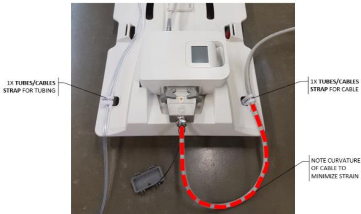
Figure 27: Tube-and-cable straps of base plate: one for tube sets and one for RF cable
