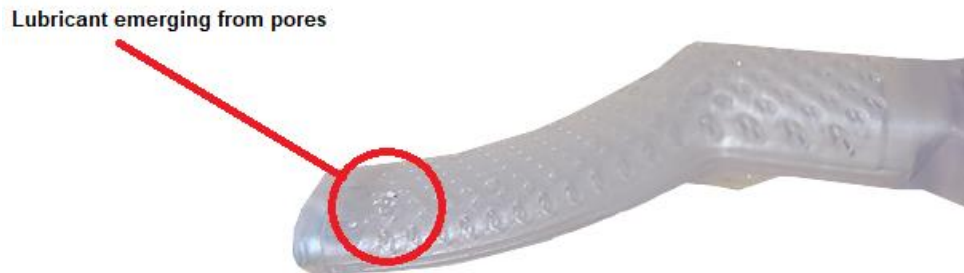
Figure 13: Lubricant emerging from ECD pores
