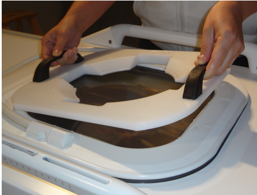
Fig. 104: Placing the QA Phantom Plate over the ultrasound window.
