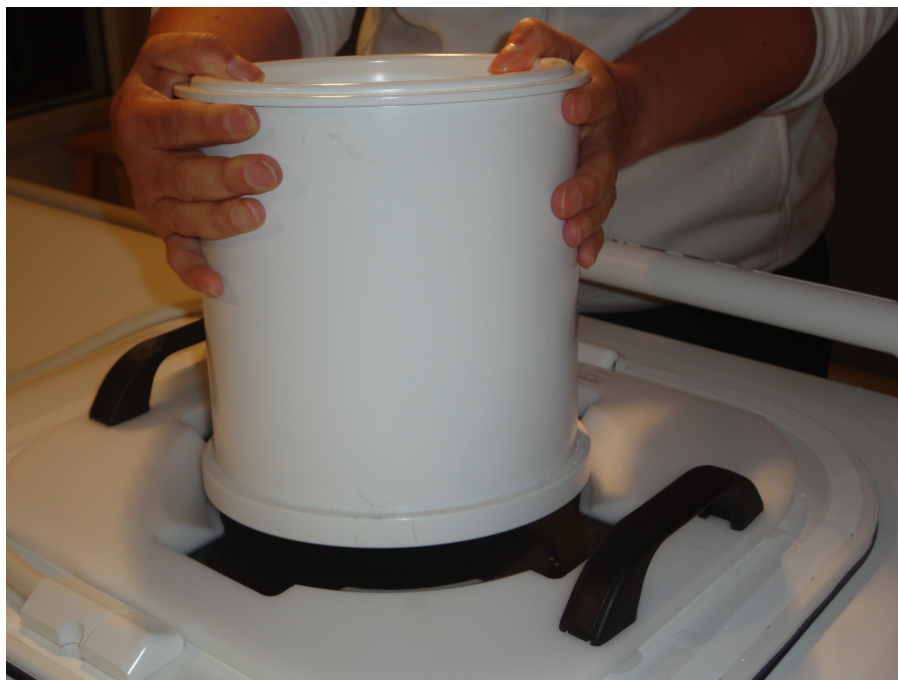
Fig. 105: Place one edge of the QA phantom on the phantom plate. Gently lower the QA phantom onto the phantom plate.
