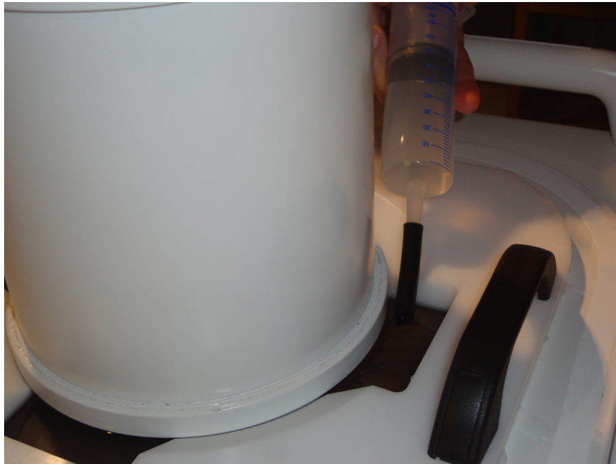
Fig. 106: Fill any remaining air pockets under the phantom with degassed water.
