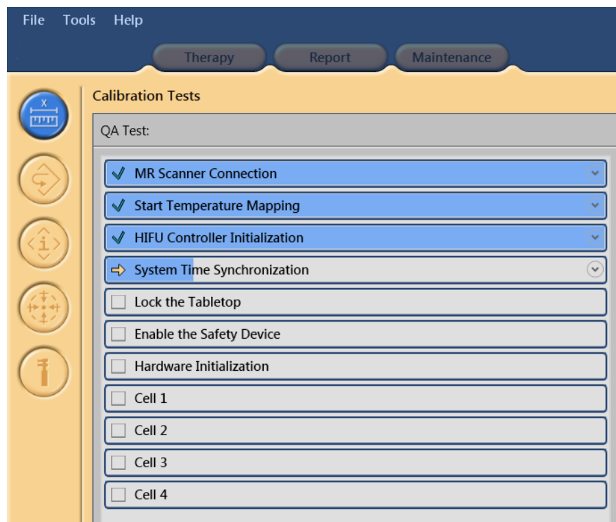
Fig. 110: Automatic QA Test has successfully passed the first three phases and is now performing System Time Synchronization.
