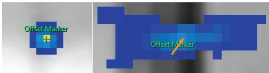
Fig. 86: If the offset marker does not appear at the center of the heating, drag the offset marker to the center of the heating manually.
