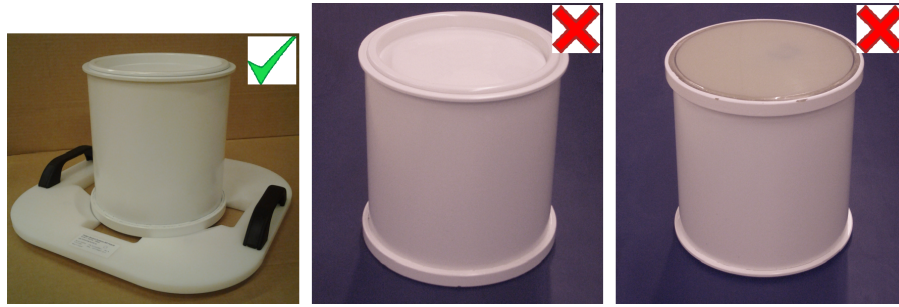
Fig. 121: Store the QA phantom on the QA Phantom Plate with the membrane facing down.
