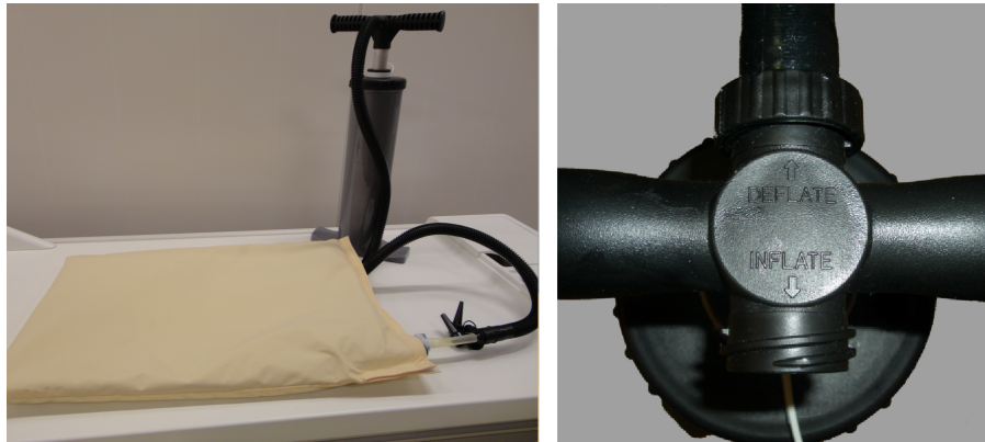
Fig. 125: Air pump. Right: Air hose connected to the Deflate side of the handle.
