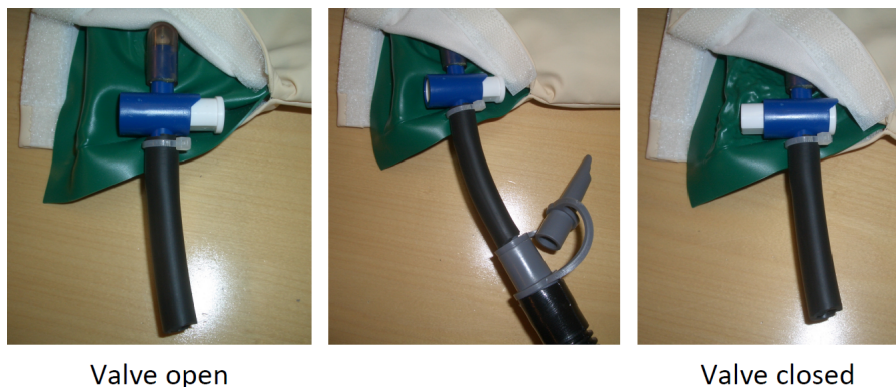
Fig. 128: Another type of valve. Left: the valve is open; middle: the air hose is connected; right: the valve is closed and the air hose has been detached.
