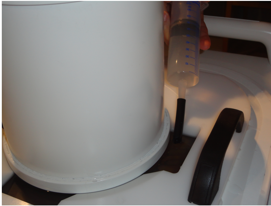
Fig. 114: Fill any remaining air pockets under the phantom with degassed water.
