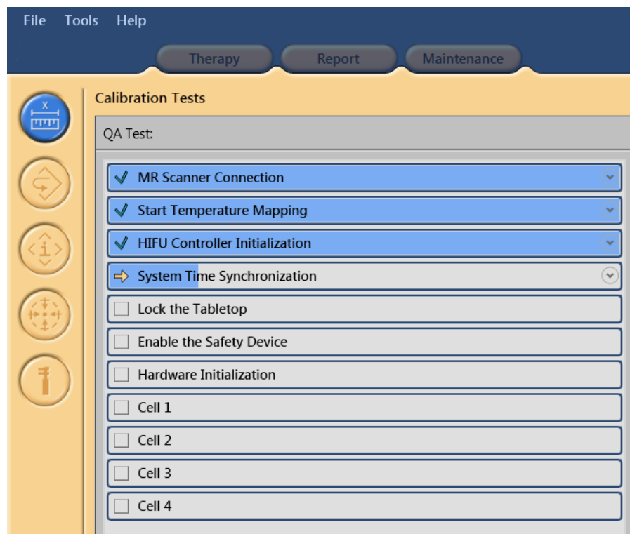
Fig. 118: Automatic QA Test has successfully passed the first three phases and is now performing System Time Synchronization.
