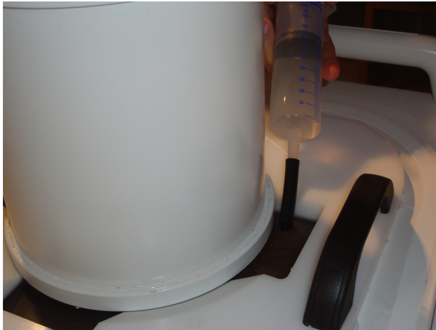
Fig. 105: Fill any remaining air pockets under the phantom with degassed water.
