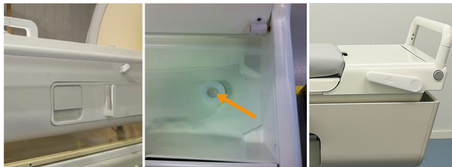
Fig. 8: Left: Table Top release handle. Middle: The emergency Table Top release button located in the accessory box. Right: The emergency Table Top release handle located on the side of the accessory box.
