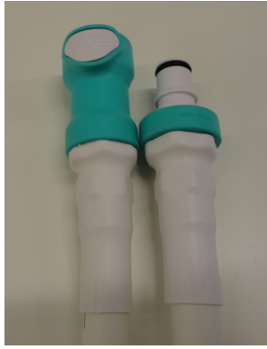
Fig. 54: Connect the two connectors in DISC hoses to the connectors in the Sonalleve Table Top.
