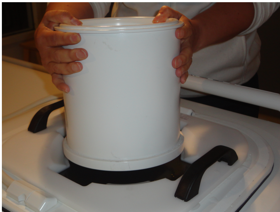
Fig. 104: Place one edge of the QA phantom on the phantom plate. Gently lower the QA phantom onto the phantom plate.
