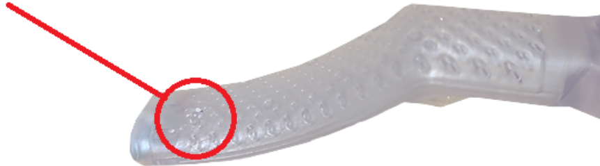
Figure 13: Lubricant emerging from ECD pores
