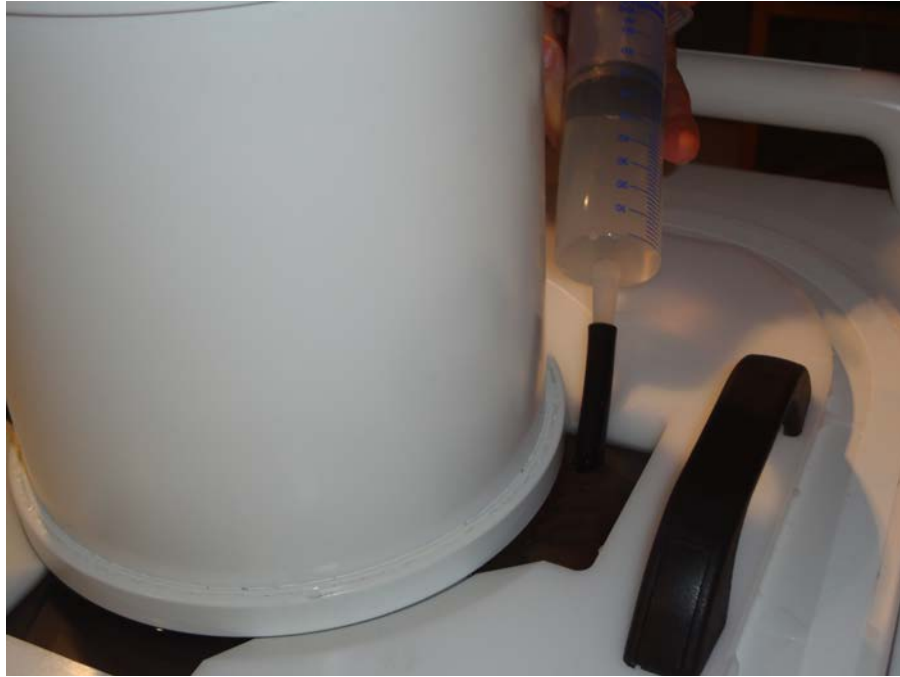
Fig. 102: Fill any remaining air pockets under the phantom with degassed water.
