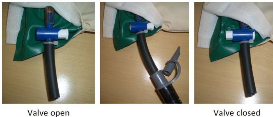
Fig. 116: Another type of valve. Left: the valve is open; middle: the air hose is connected; right: the valve is closed and the air hose has been detached.
