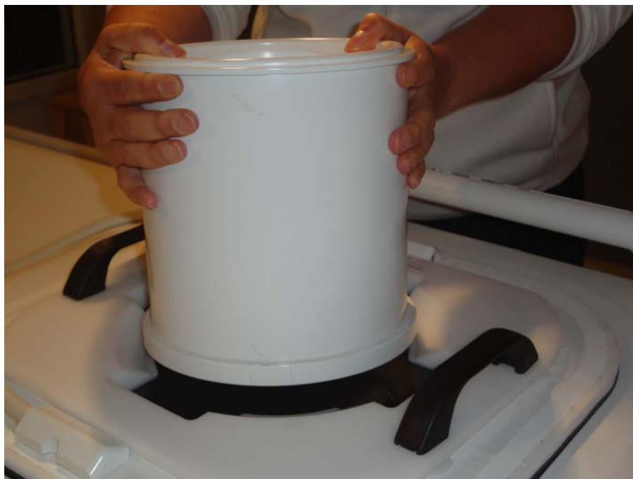
Fig. 101: Place one edge of the QA phantom on the phantom plate. Gently lower the QA phantom onto the phantom plate.
