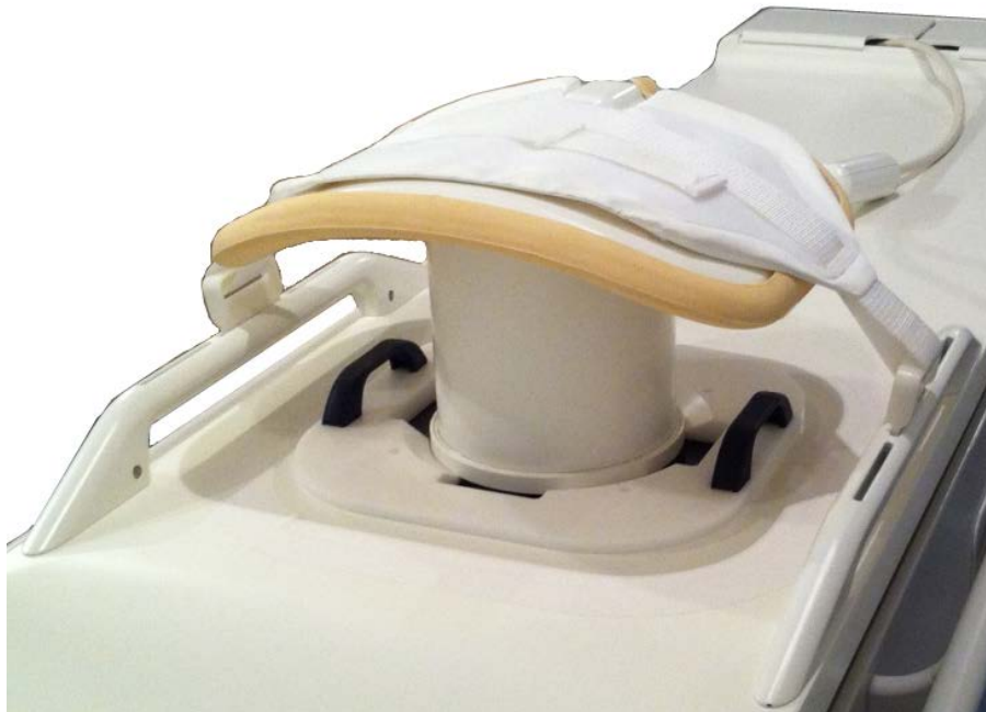
Fig. 103: QA phantom ready for sonication.
