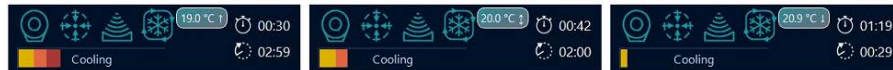
Fig. 17: Three examples of cooling time in the System Status Display. Left: Almost one third of the remaining system-recommended cooling time is mandatory and cannot be overridden. Middle: The cooling period can be overridden because there is no mandatory cooling time, but the system indicates a high risk of internal burn. Right: Recommended cooling time still remaining, but it is possible to use the override and start sonication.
