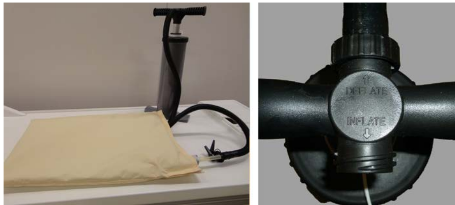
Fig. 113: Air pump. Right: Air hose connected to the Deflate side of the handle.
