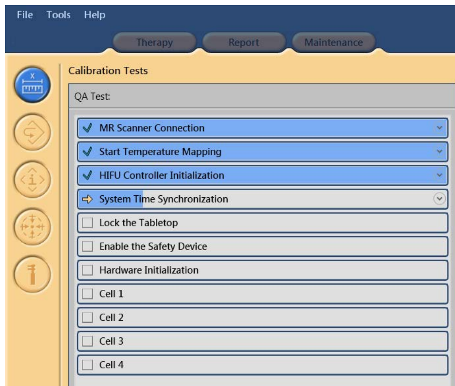
Fig. 106: Automatic QA Test has successfully passed the first three phases and is now performing System Time Synchronization.
