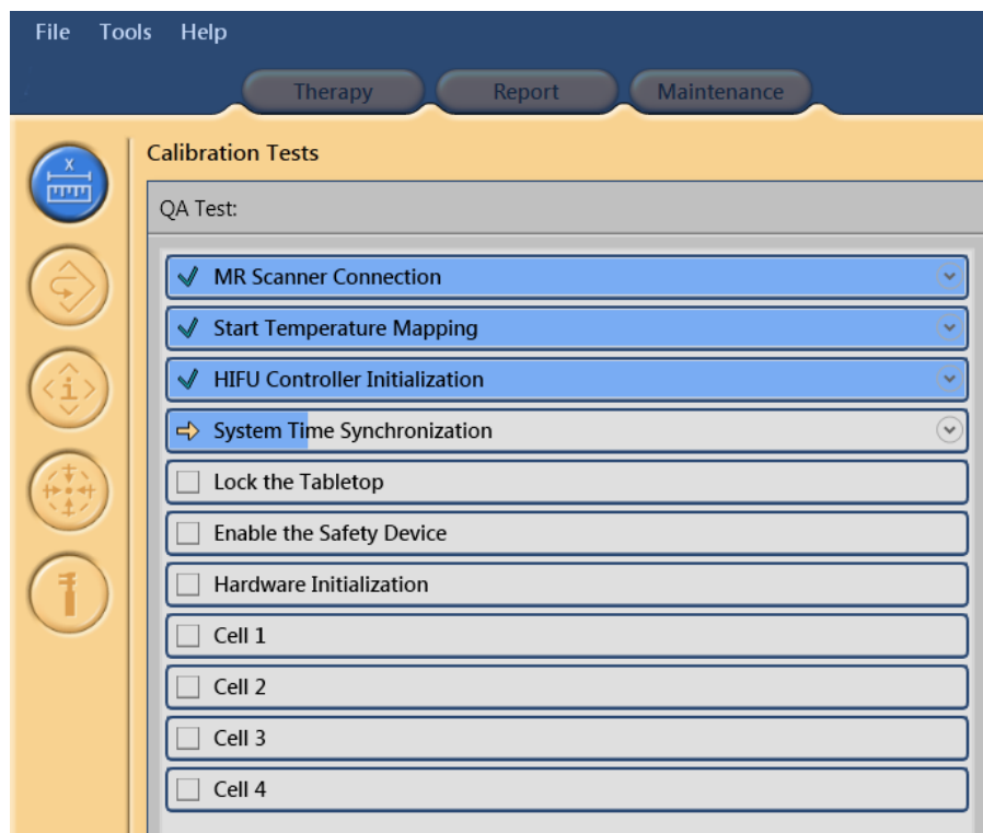
Fig. 112: Automatic QA Test has successfully passed the first three phases and is now performing System Time Synchronization.
