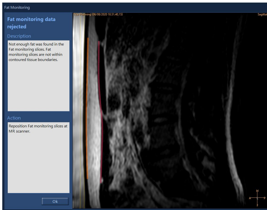
Fig. 38: The Fat Monitoring dialog shows the position of the T2 fat monitoring scan with respect to tissue boundaries. It also provides more information on why the fat monitoring data could not be used. The image can be windowed using the standard tools.
