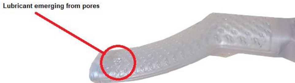
Figure 12: Lubricant emerging from ECD pores
