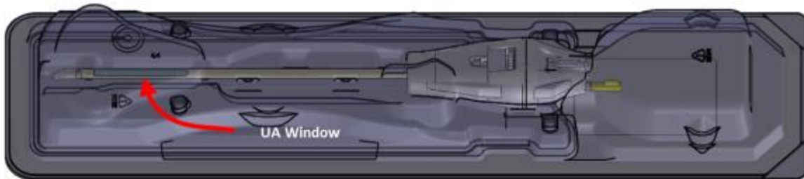
Figure 10: Examine the UA window for air bubbles
