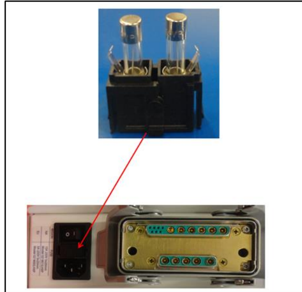
Figure 14: Fuse drawer placement
