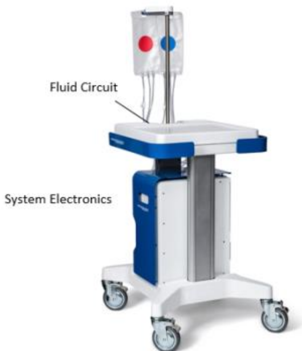
Figure 1: System Cart and components
