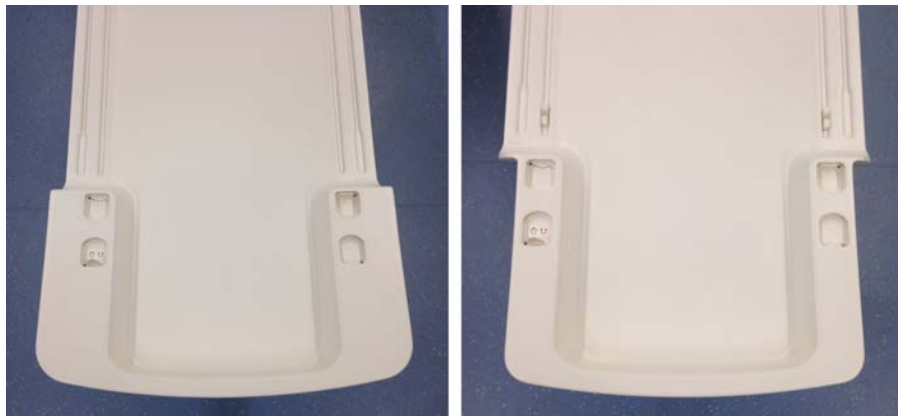
Fig. 53: Left: This type of Ingenia thin tabletop needs to be removed before the Sonalleve Table Top can be placed in position. Right: The narrower end in this type of Ingenia thin tabletop allows the Sonalleve Table Top to be placed in position without removing the Ingenia thin tabletop.
