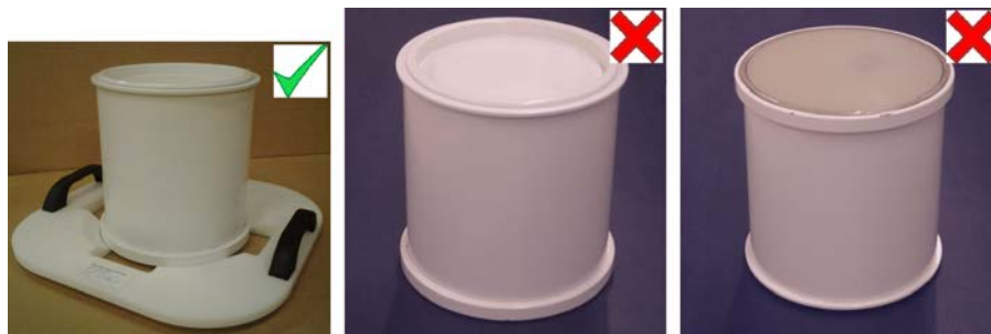
Fig. 115: Store the QA phantom on the QA Phantom Plate with the membrane facing down.
