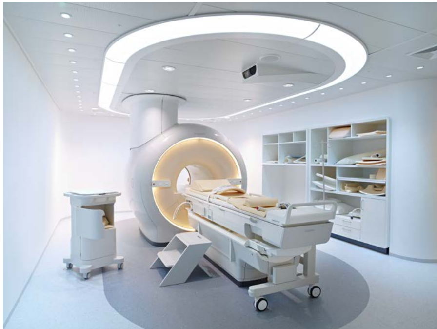
Fig. 3: Sonalleve Patient Table docked to the scanner.
