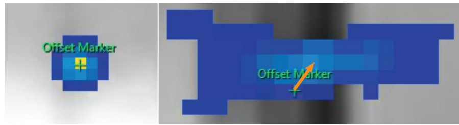
Fig. 90: If the offset marker does not appear at the center of the heating, drag the offset marker to the center of the heating manually.
