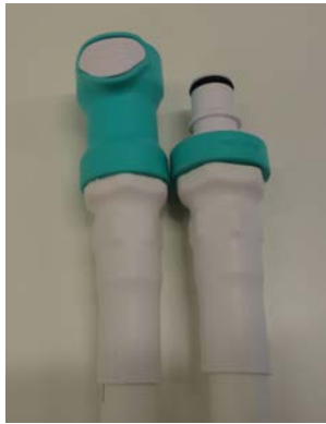
Fig. 56: Connect the two connectors in DISC hoses to the connectors in the Sonalleve Patient Table.
