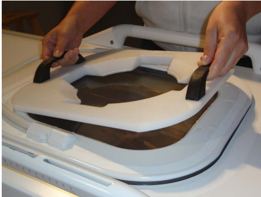
Fig. 106: Placing the QA Phantom Plate over the ultrasound window.
