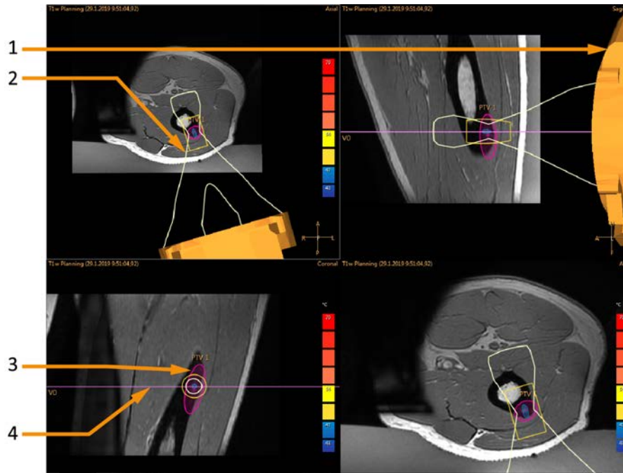
Fig. 36: Overlays on top of the transducer view: Transducer overlay (1), Transducer beam overlay (2), PTV overlay (3), View slice overlay (4)
