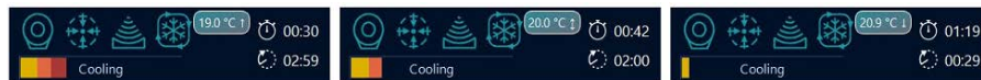
Fig. 22: Three examples of cooling time in the System Status Display. Left: Almost one third of the remaining system-recommended cooling time is mandatory and cannot be overridden. Middle: The cooling period can be overridden because there is no mandatory cooling time, but the system indicates a high risk of internal burn. Right: Recommended cooling time still remaining, but it is possible to use the override and start sonication.
