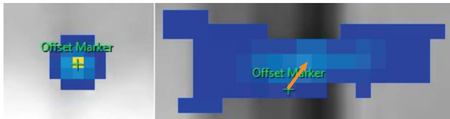
Fig. 94: If the offset marker does not appear at the center of the heating, drag the offset marker to the center of the heating manually.
