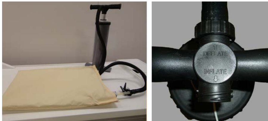
Fig. 123: Air pump. Right: Air hose connected to the Deflate side of the handle.
