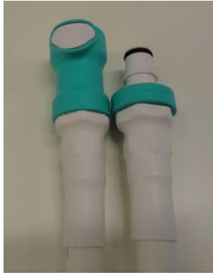
Fig. 57: Connect the two connectors in DISC hoses to the connectors in the Sonalleve Patient Table.
