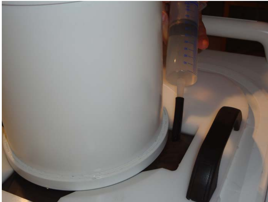
Fig. 112: Fill any remaining air pockets under the phantom with degassed water.
