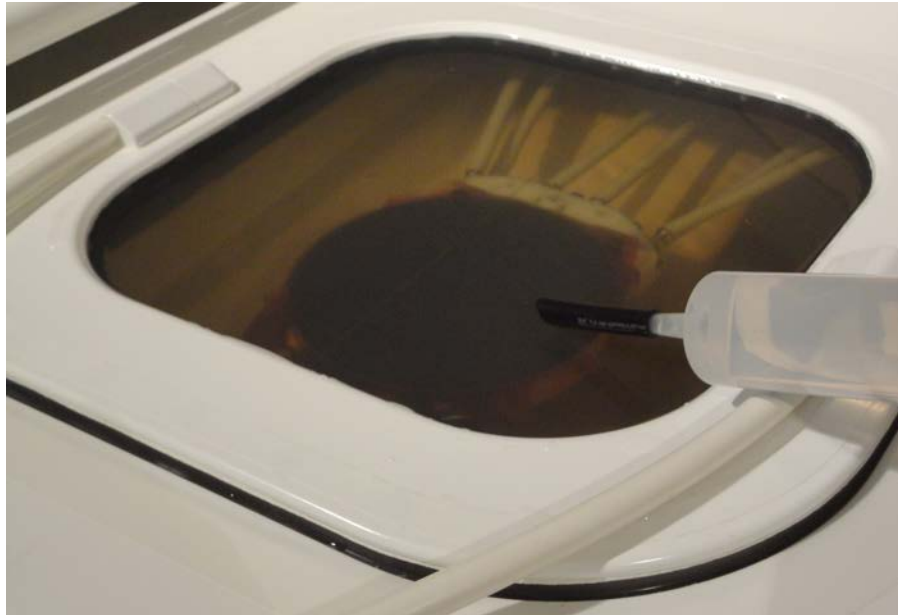
Fig. 108: Preparing the Sonalleve Patient Table with degassed water for phantom.
