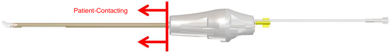
Figure 12. Patient-contacting region of the UA
