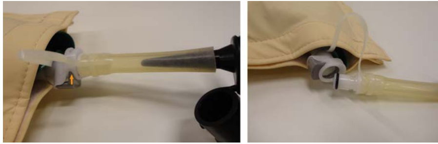
Fig. 129: Releasing the tube from the valve.
