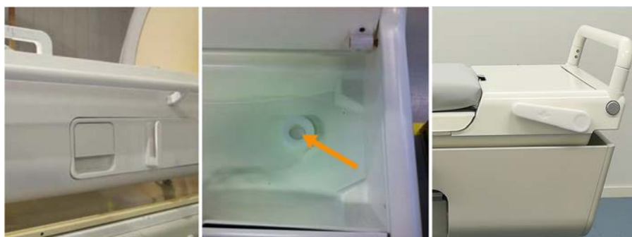
Fig. 9: Left: Table Top release handle. Middle: The emergency Table Top release button located in the accessory box. Right: The emergency Table Top release handle located on the side of the accessory box.
