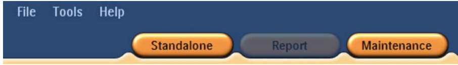
Fig. 29: The application selection buttons when Standalone is selected in the start page of the Sonalleve MR-HIFU application. To start in the Standalone mode, click Standalone .
