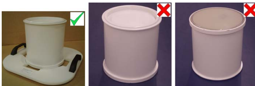
Fig. 123: Store the QA phantom on the QA Phantom Plate with the membrane facing down.
