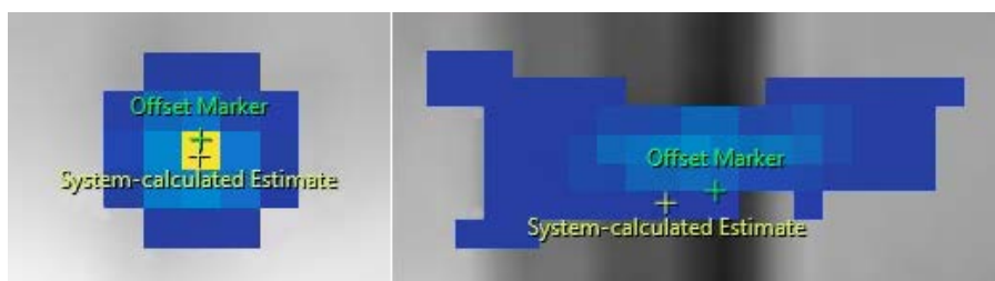
Fig. 91: When you move the offset marker, another marker appears at where the system-calculated estimate was.
