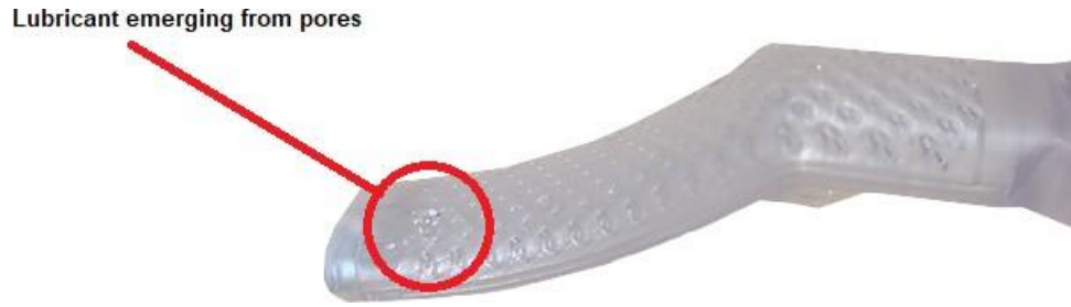
Figure 18: Lubricant emerging from ECD pores
