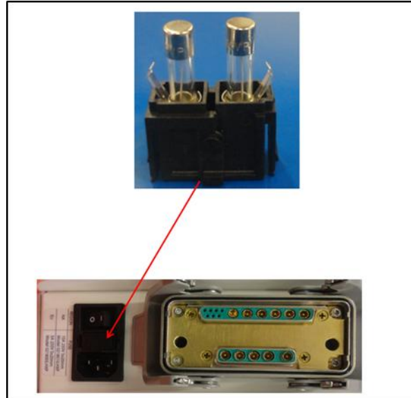
Figure 14: Fuse drawer placement
