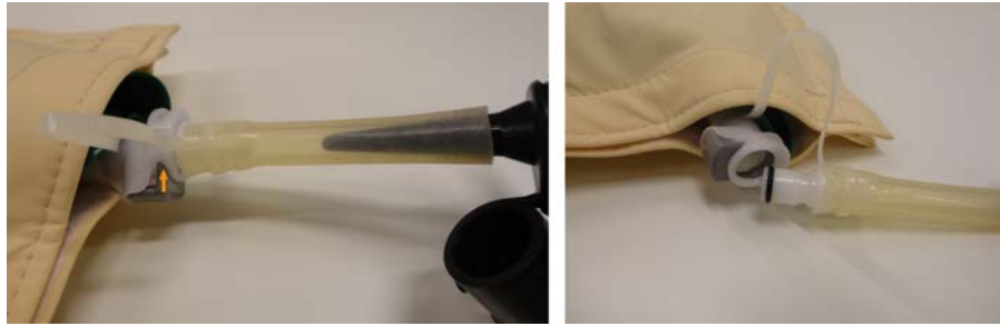
Fig. 121: Releasing the tube from the valve.
