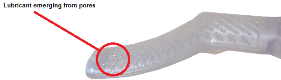
Figure 18: Lubricant emerging from ECD pores
