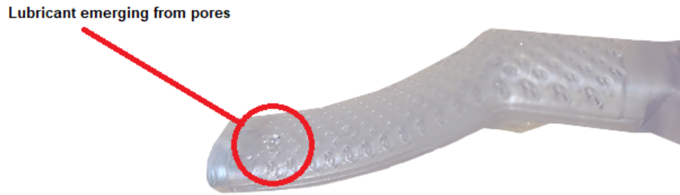
Figure 17: Lubricant emerging from ECD pores
